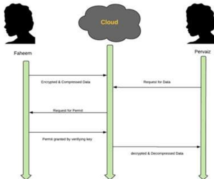
**Figure 12.** Sequence diagram of protected sharing.
